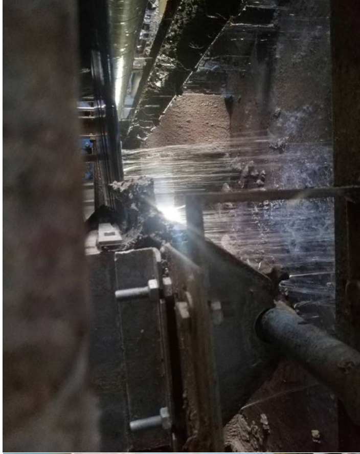
Process cleaning belt by reuse water
